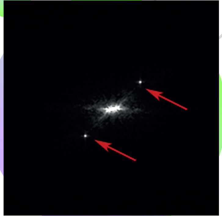
Fig. 2D demonstration of peak points in a noisy image's amplitude spectrum.
